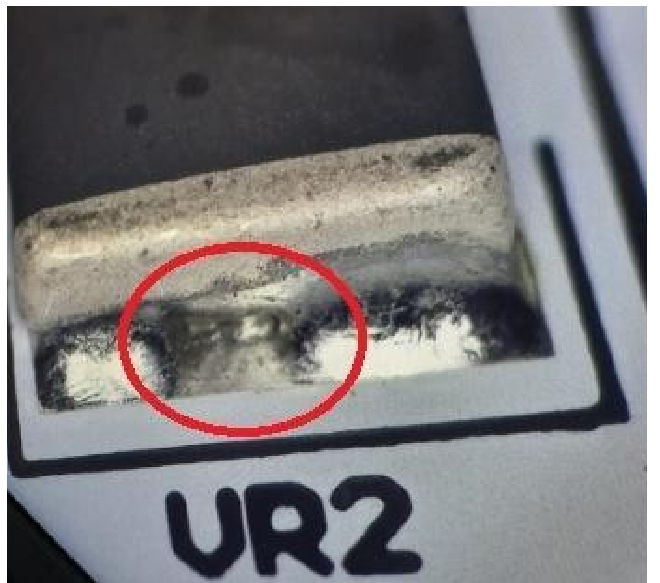
Termination height-3 mm (Half solder)
